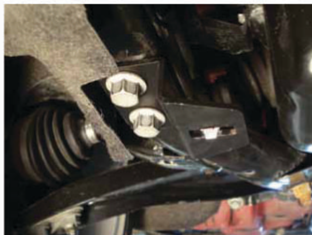
Step 2 - Remove the (2) Subframe bolts on each side of the car and install the skid plate brackets as shown above. Note: Work on one side of the car at a time.
