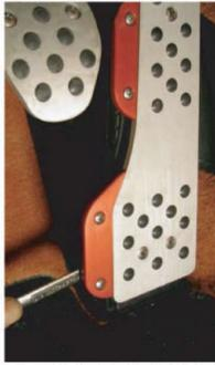
Lock pedal cover into desired position by tightening the (3) nuts on the back of the pedal cover using a 3/8" wrench.
