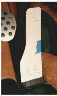
Cut out the supplied template and place over the top of the factory pedal in the desired position and attach with tape.
